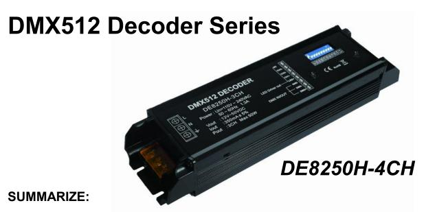
Thank you for using DMX512 Decoder series. It adopts the advanced micro-computer control technology, it converts the DMX-512/1990 standard digital signal adopted widely in international to the analog control signal. Output 1~3 Channels for option and each channel able to achieve 256 levels of brightness controlling, and also it can be used as the connector of PC digital-light controller and analog light modulator. It is mainly used for the controlling of buildings & lights applied LED.
